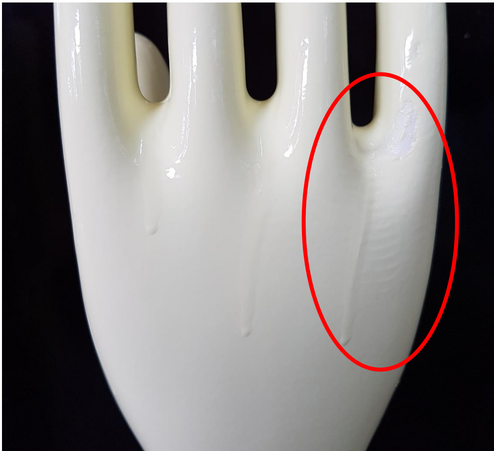
Uneven wetting with obvious flow mark.
