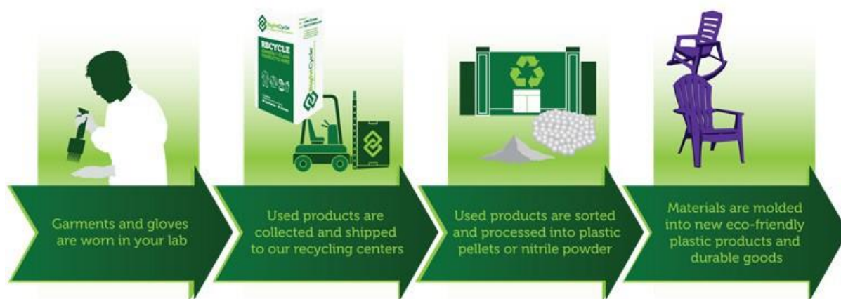
Figure 1 : Nitrile glove recycling conceptual diagram flow 2
